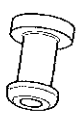
8 END CAP W/ MONOLITHIC SCREW SLEEVE N.T.S. (LEFT SHOWN, RIGHT IS MIRROR) RIGID NYLON, 76-78 TYPE 'O' SHORE HARDNESS
